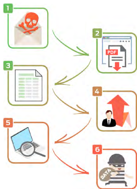
Figure 1. A typical attack starts with an initial contact and progresses through various stages, including reconnaissance, stealing data and causing damage.
